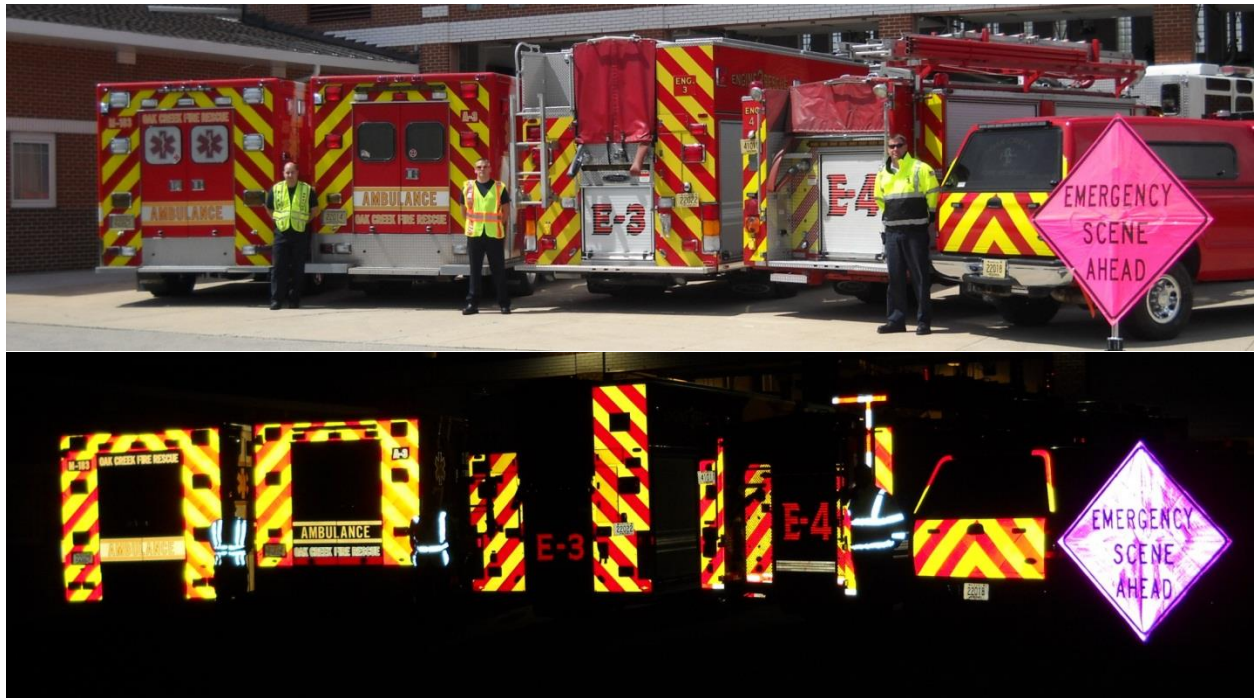
Figure 4: Emergency Vehicles with Retroreflective Chevron Striping (Photo Courtesy of the City of Oak Creek Fire Department, WI)
